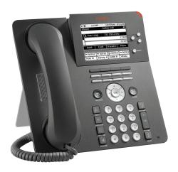
managing multiple calls and dropping conference call participants. The 9650 supports built-in button module functionality (8 physical buttons with shift capability for a total of 16 feature keys) to provide simple one-touch access to partners, speed dials and feature keys. And, with its dual position flip stand, the 9650 makes a smart looking addition to any desk.
